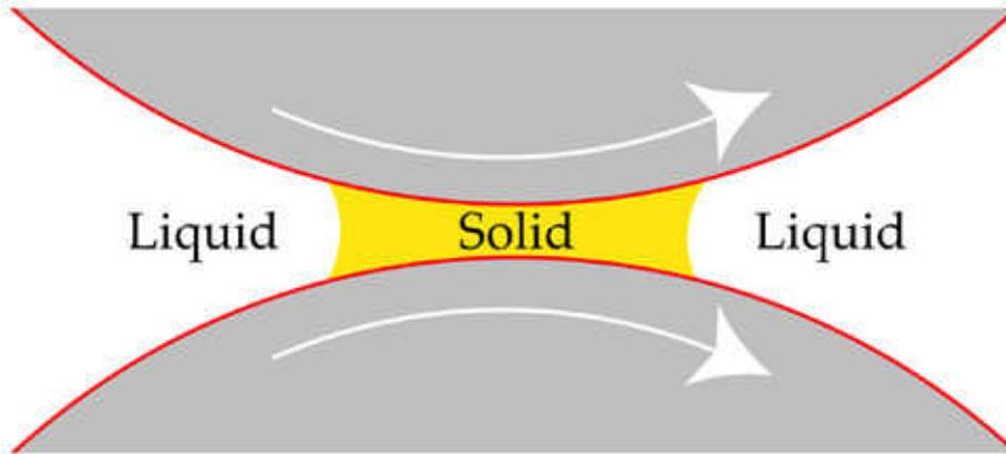
Figure 1 EHD lubricants turn into a glassy solid for a few microseconds under the high forces present in a CVT. This momentary solid state prevents metal-to-metal contact and greatly increases traction.
