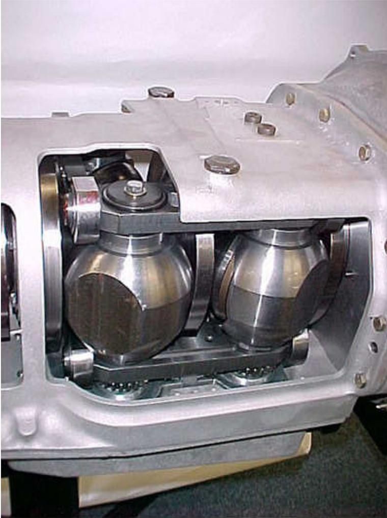
Figure 3                      Cut-away view of a continuously variable transmission (CVT) under development at Transmission Technologies Corporation.
