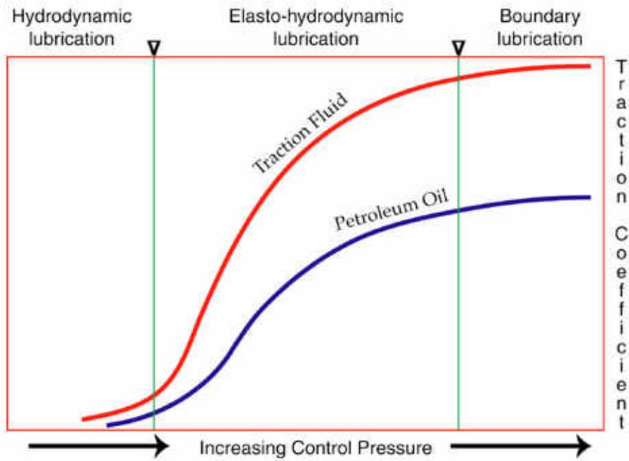
Figure 2 A comparison of behavior of petroleum-based lubricants and synthetic EHLs under increasing pressure. EHLs have a higher traction coefficient across the range of pressures.
