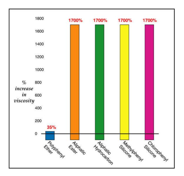
Figure 1 Increase in viscosity of various lubricating chemical classes after exposure to  $10^{11}$  ergs/gram (equivalent to  $10^{9}$  rads) of electron radiation.
