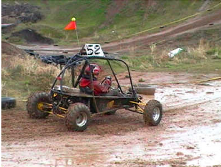
Figure 2 Team 52's vehicle sails through the endurance portion of the Mini-Baja. For maximum efficiency, engine rpms were kept constant, while speed was varied by the IVT/CVT and its liquid/solid transmission fluid.
