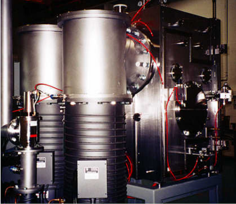
Figure 4 Vacuum diffusion pumps in operation, here in a vacuum coating operation. [Photo courtesy of Mill Lane Engineering]
